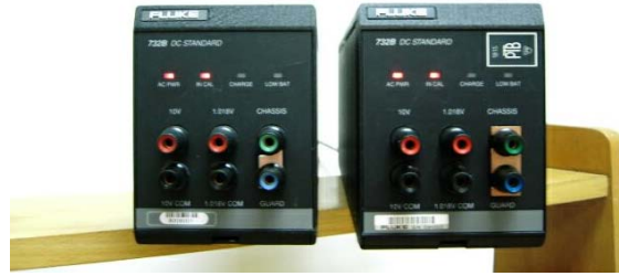
Fig. 1 Etaloane de tensiune tip Fluke 732B cu diodă Zener Fig.1 Fluke type of 732B Zener voltage standards
